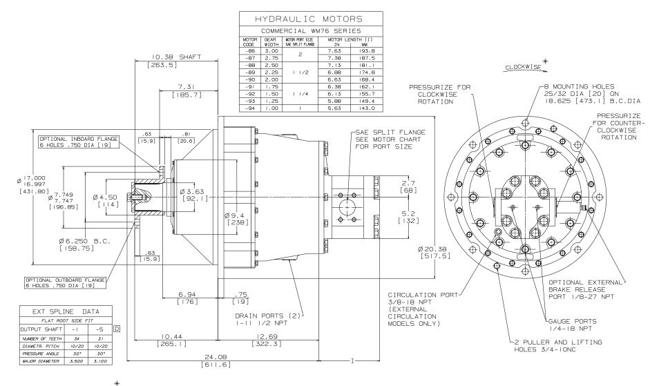
NOTE: - CLOCKWISE & COUNTER-CLOCKWISE OUTPUT SHAFT ROTATION IS ESTABLISHED BY LOOKING AT THE HYDRAULIC MOTOR
