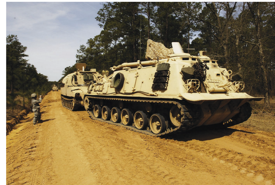
ARMORED PERSONNEL CARRIERS TESTING RECOVERY WINCHES
