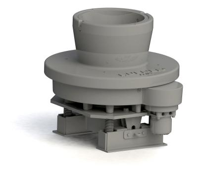
The Rotating Mousehole (RMH) sits on the rig floor to allow the drill pipe to be readily available when needed. The RMH increases the drilling efficiency by enabling users to rotate and join 3 sections of pipe instead of one section at a time.
